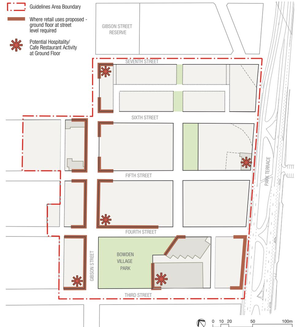
FIGURE 13: Required Ground Floor at Street Level Location Plan
