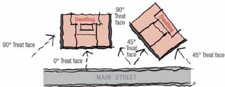
FIGURE 41: Determination of treated facades
