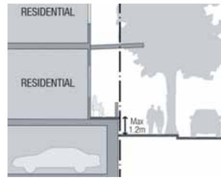
FIGURE 35: Maximum height of semi-basements above finished street level
