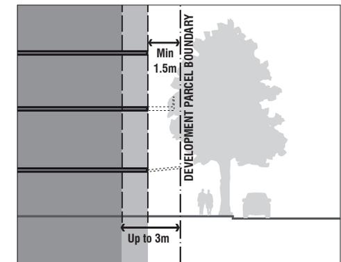
FIGURE 21: Min 1.5m up to Max 3m Street Setback Section
