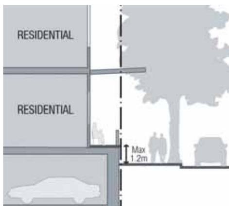
FIGURE 14: Maximum height that ground floor may be raised above finished footpath level
